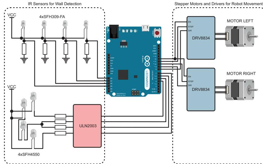
Fig. 2: Micromouse kit block diagram.
