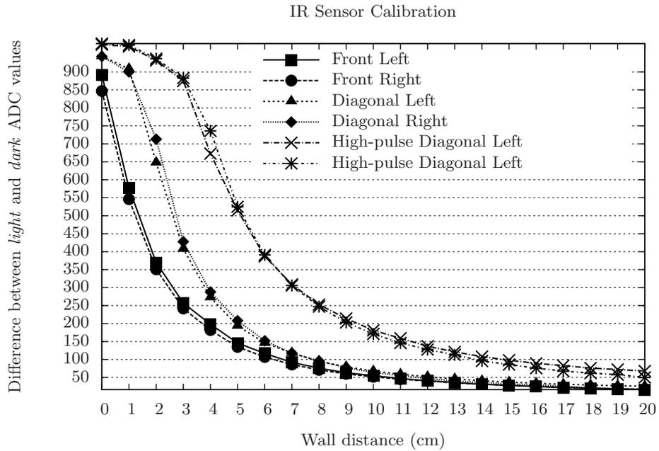
Fig. 4: Infra-red sensor calibration curve.
