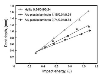
Fig. 6. Dynamic dent resistance of some aluminium plastic laminates.
