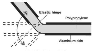
Fig. 3. Elastic hinge of Hylite.
