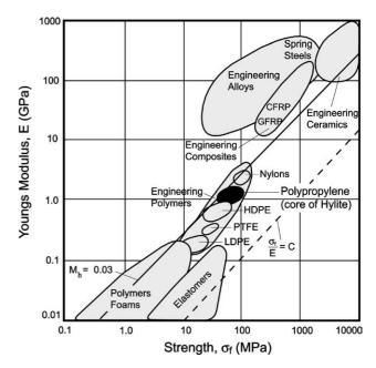
Fig. 4. Materials for elastic hinges [7].
