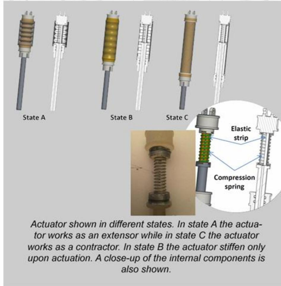
*Actuator shown in different states. In state A the actuator works as an extensor while in state C the actuator works as a contractor. In state B the actuator stiffen only upon actuation. A close-up of the internal components is also shown.*
