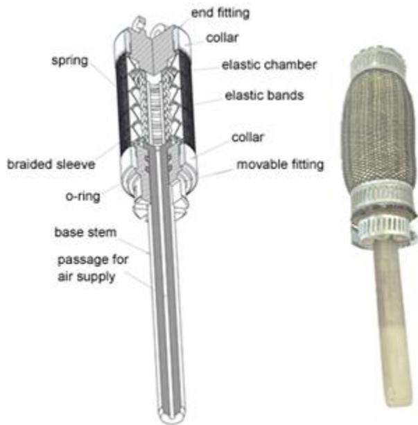
*Actuator design schematics. Physical prototype and sectioned CAD rendering.*
