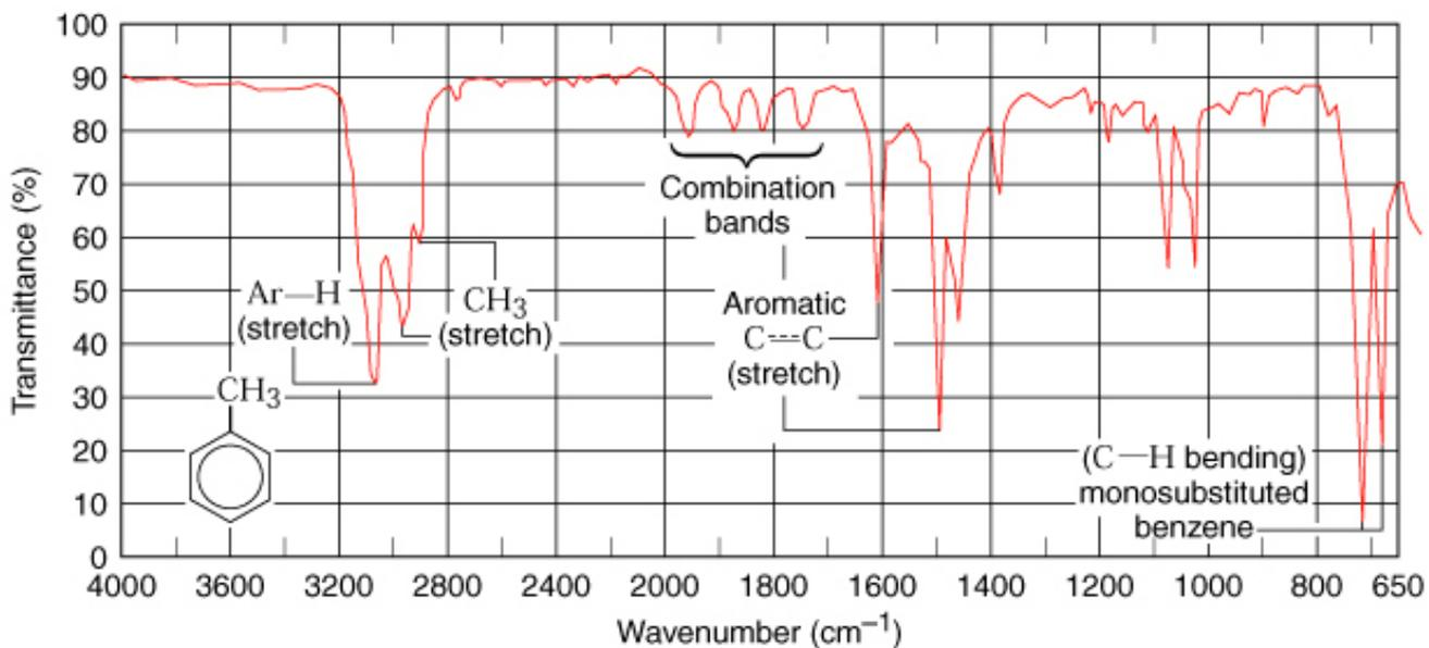
Figure 2.12 The IR spectrum of methylbenzene (toluene).
