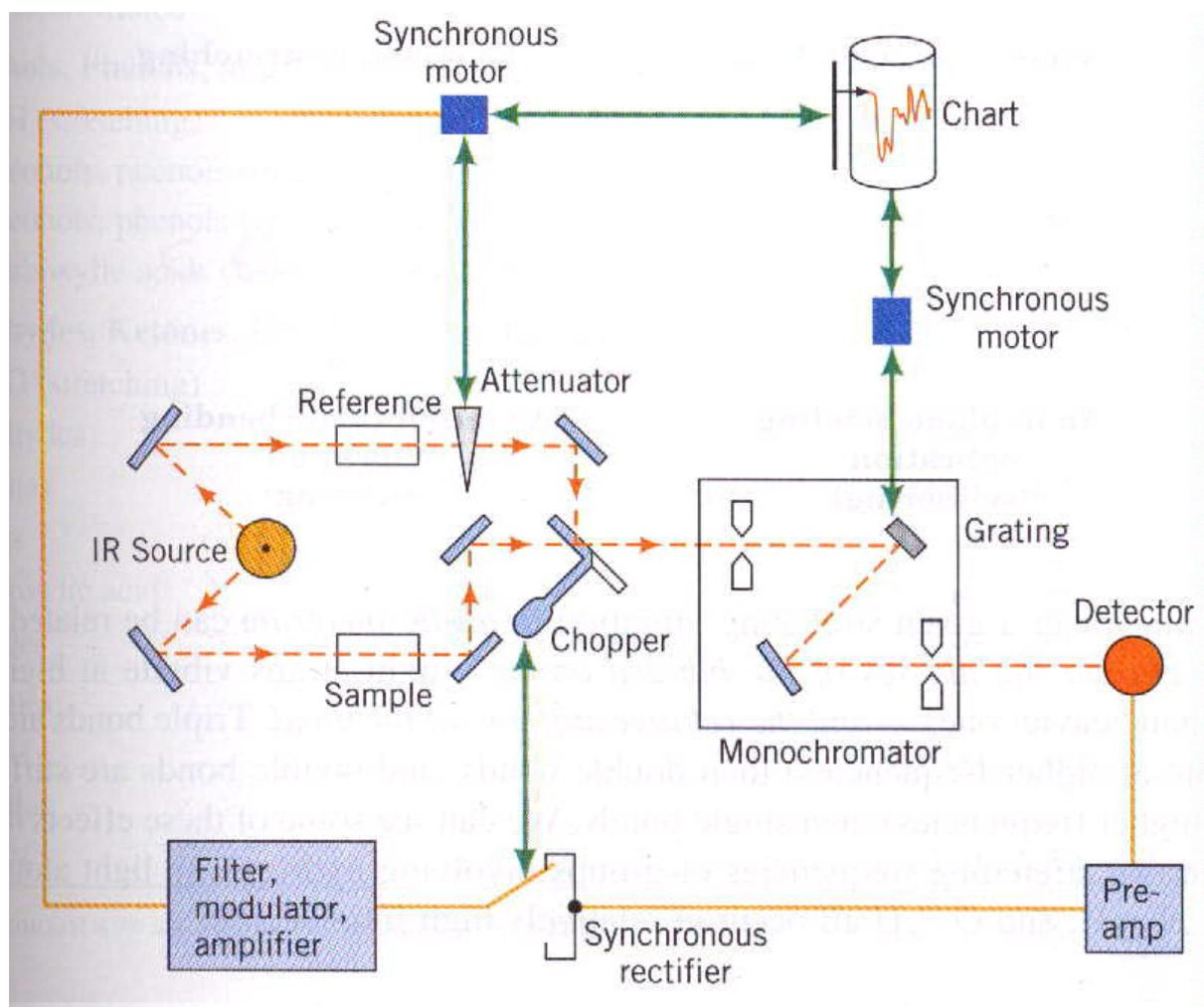
**Figure 2.10** Diagram of a double-beam infrared spectrometer. [From Skoog D. A.; Holler, F. J.; Kieman, T. A. *principles of instrumental analysis*, 5th ed., Saunders: New York, 1998; p 398.].
