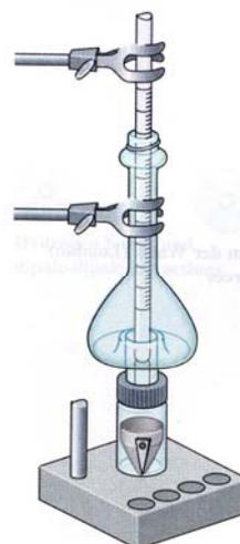
**An instrument used to measure melting point.**      **A microscale distillation apparatus.**
