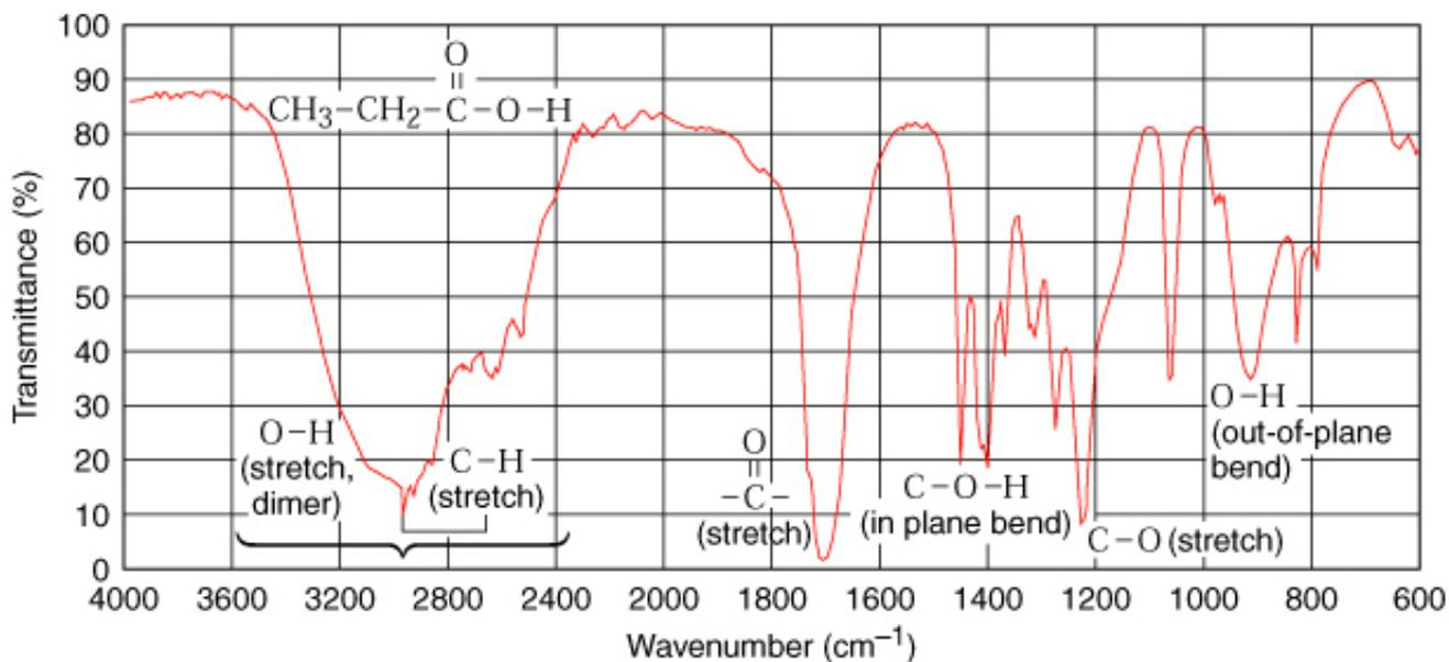
Figure 2.16 The infrared spectrum of propanoic acid.
