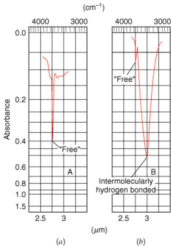
Figure 2.15 The IR spectrum of cyclohexanol .
